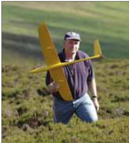
John McConville seems less than happy with his attempts to sort out the constant glitching, which plagued previous 'Microfloh' owner Mike Pirie. A change of rx solved the problem.
