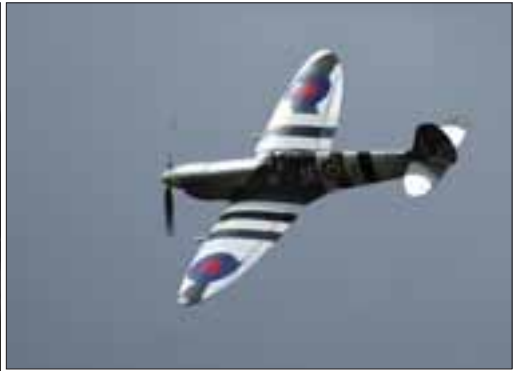
Stunning photo of a Ripmax 'Spitfire' straffing ADS members' cars ...shame about the folding prop though! Impressive performance from Roger Taite's 10 cell, brushless powered model. 48" span, 1695g AUW, Hacker B50-9S/6.7:1 box turning a cut-down (to 13") Aeronaut 14x10 fed by a 1950mAh nimh pack. Cannons added to this Mk.IX version in Wing Cdr Jonnie Johnson's personal markings. 3S lipo packs under investigation to drop the weight a tad.
