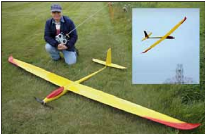
Abby and 'Excalibur'. A superb 3m electric soarer. Hacker B50-10S with 6.7:1 gearbox, a Jeti 70A esc, 12x2400 nicad pack, 15"x13" prop, 6 Hitec HS125MG servos.
