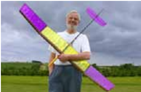
JB gets around to HLG's at last. Model is a 'Pearl', available from Guy at SoarHigh Models. Don't be deceived by the flimsy appearance (of the model, that is). It's designed to be discus launched, an entertaining alternative to mini-bungee use or straight javelin throws if you're on first name terms with your local A&E, so the airframe is mainly carbon and outstandingly strong.
