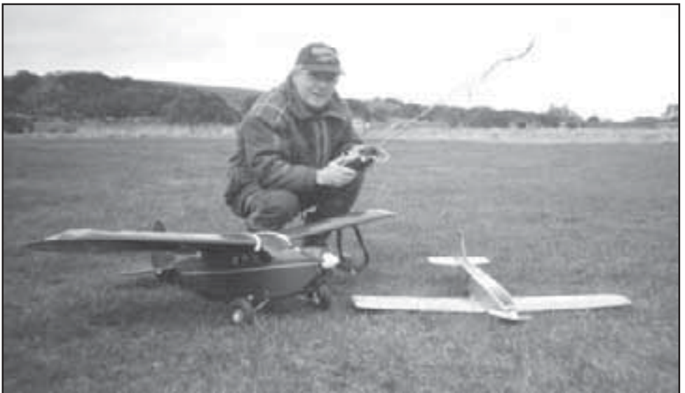
Quietly enjoying a high degree of success with electric models, George Thomson with the dinky little Tiger Shark and what looks like a cross between a Lazy Bee and a Junior 60, the vintagesque Magpie. You've probably guessed, yet another Speed 600 motor, this time with an 8 cell 2100 Nicad pack making up the powertrain.
