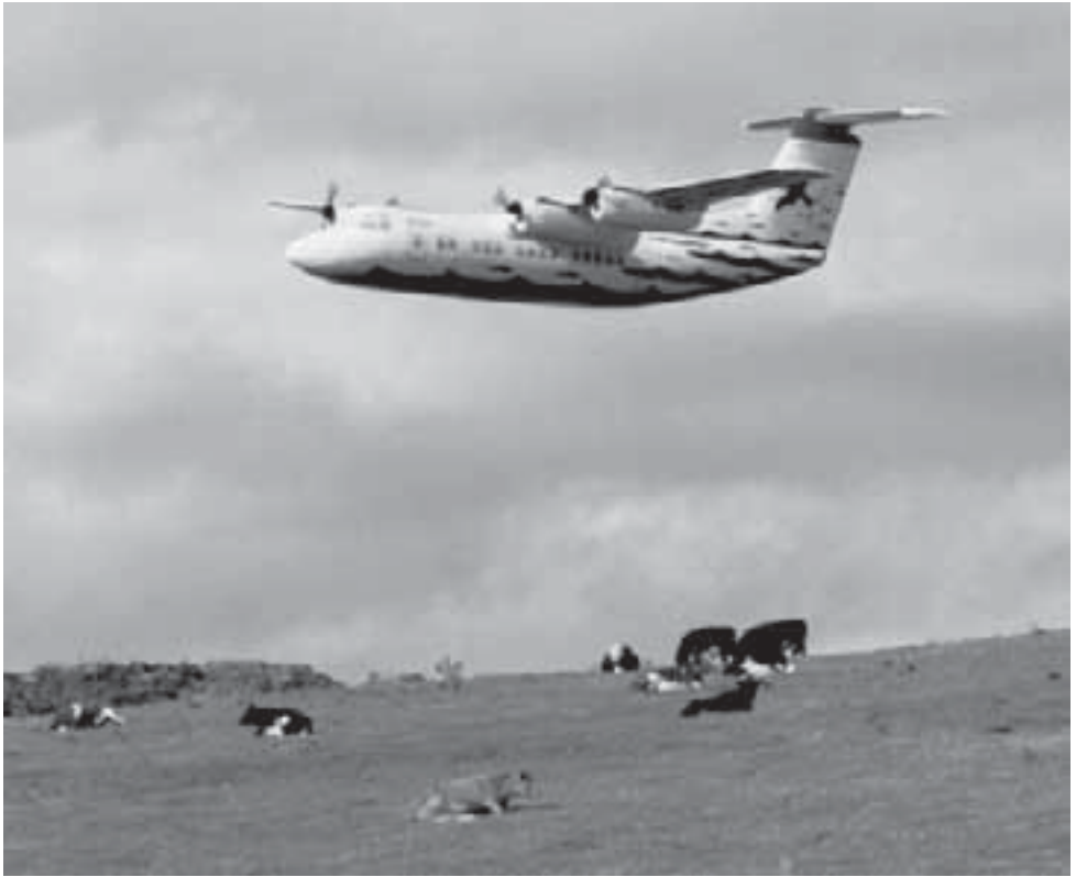
A Dash 7 buzzes Calder Park. The Robbe kit with four Speed 400 motors, fed by an 8 cell, 2400 Nicad pack. The cows in the next field were unimpressed! (photo: Mike Pirie)
