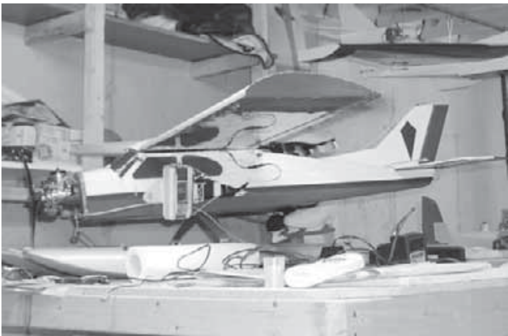
The camera plane. Just shows what can be done with a straightforward compact camera installation. Also note that the model for such ventures doesn't have to be a big one. Just mount all the sensitive bits on the opposite side to the exhaust, otherwise you may have trouble explaining to momma why her camera appears to be covered in body lotion.
