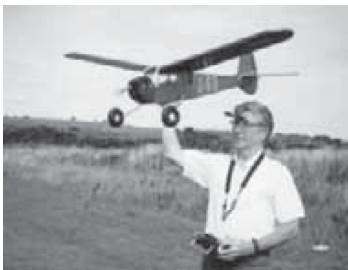
You just can't keep this guy away from the glue at the moment! George Thomson, a man of substance(s), about to launch his Junior 60. Unlike Dave Curry's version, this one uses a cheap 'n' cheerful belt driven speed 600 motor, fed by an 8 x 2100 pack. (groovy 'shades' by the way, George!)
