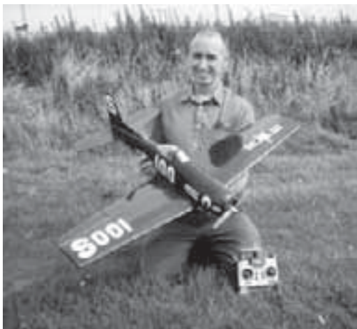
Performing his world famous Toulouse-Lautrec impression, Alan Stewart poses with a fine example of the Balsacraft Bearcat. Seven cells driving a speed 600 motor.
