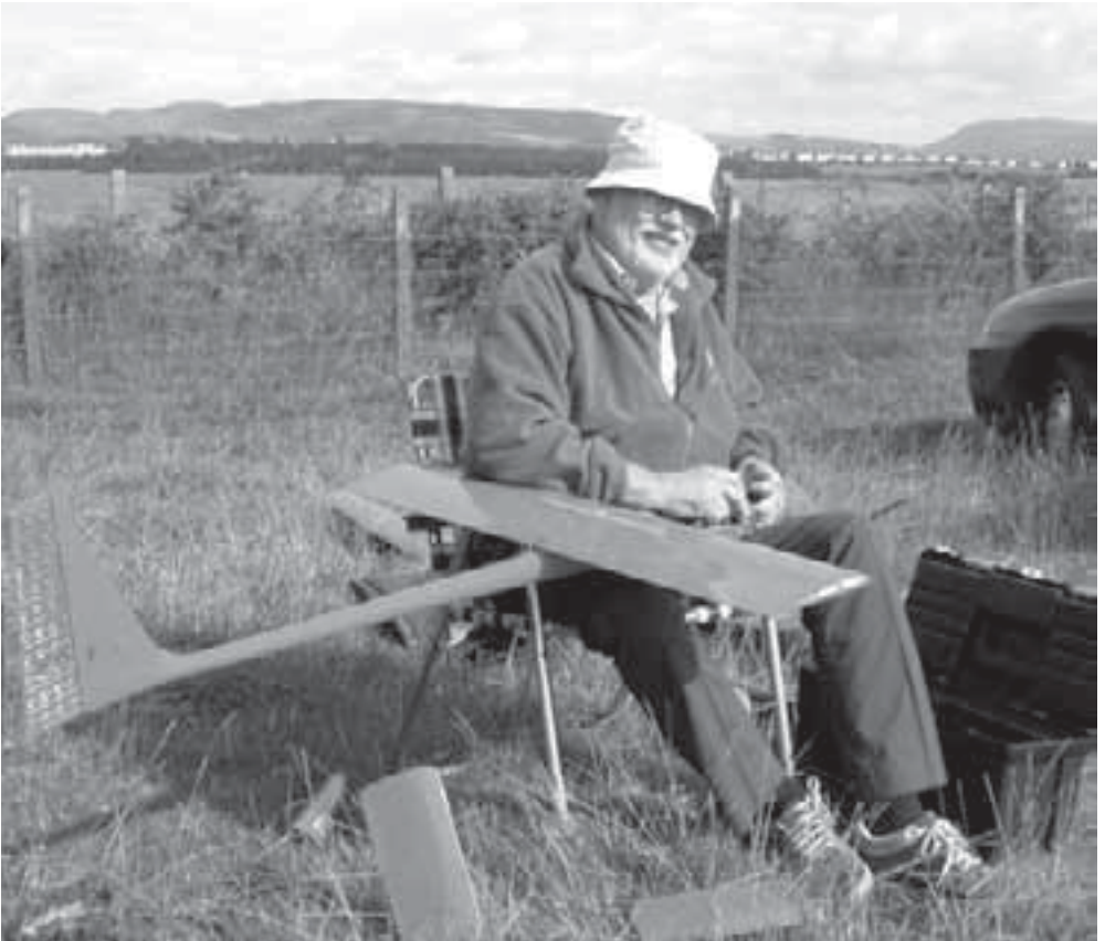
Al Wisher preparing for 100S, having just disconnected the hoses from the helium tank after pressurising the sealed wings and fuz
