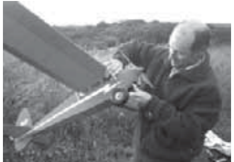
Dave Curry's impressive slow fly Junior 60, powered by a 12 volt belt driven speed 600 motor. A generous wing area ensures that it remains airborne for hours (well, a long time!), running off a 10 x 1000 mAh battery pack. Dave explained to me that it was an old Ben Buckle design that dates back to the days when he had hair, which came out far easier than this battery pack did!
