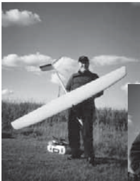
The unusual sight of George Whelan sporting a manufacturer's kit? In this case, it's a Multiplex Lucky, a 1.9 mtr slope aerobat with a RG 15 wing section. Not many V tailers in the club! After winch launching, the Lucky proved to be very fast and a tad responsive. George intends to take it to the slope to get the mixing sorted out before venturing onto the winch again!
