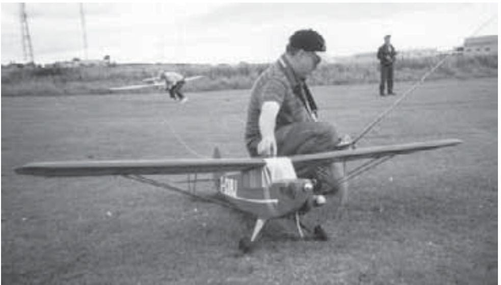
Aerotows for all. DB Cub, old ASP .75 swinging a 14x6 prop, highly reliable combo seems to launch just about anything.
