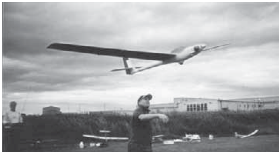
John McConville launching a 3m Wik Condor on its maiden flight. John Barnes has had this kit hidden in the loft since the old King was alive. Finally completed to help flight training of new members. Very quiet OS .26 4st. engine coupled to a 6oz tank gives c. 1 hour flight times. Generous dihedral makes for a very stable, well-mannered ship. If only JB didn't fly Mode 1...
