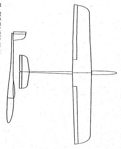
The ELIMINATOR SR (slope racer) is designed to suit the new 60" pylon racer class, but also makes a great sports aerobatic model with the RG 15 wing section giving it a good soaring performance. It flies equally well with either a standard or vee tail.
