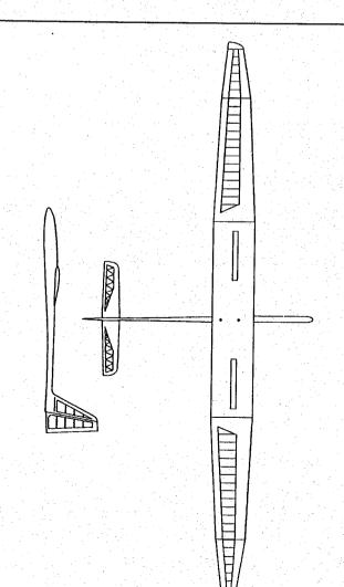
The Eliminator 134 lightweight thermal soarer features traditional wood construction. It is a top performer suitable for open class or F3J competitions, as well as the sports flyer. With its smooth, steady handling and light wing loading (9oz per sq ft) it is able to exploit those tight, light thermals. The bolt on three piece wing has a modified E193 section. Strong construction makes it ideal for fast towing or bungee launching. It has room for standard radio.
