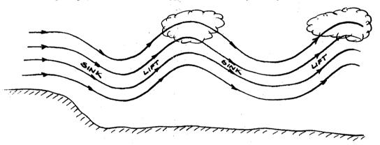
Wave can extend many miles downwind of the hill that caused it, and gliders using the rising part of the wave can experience rates of climb of over 10 knots (1000 ft/min) and can reach heights of over 30,000ft. Flights of 15,000 to 20,000ft are common at Aboyne, and having personally experienced a flight to 10,400ft in the incredibly smooth air which is typical of wave, I can only say that it was a fantastic experience.
